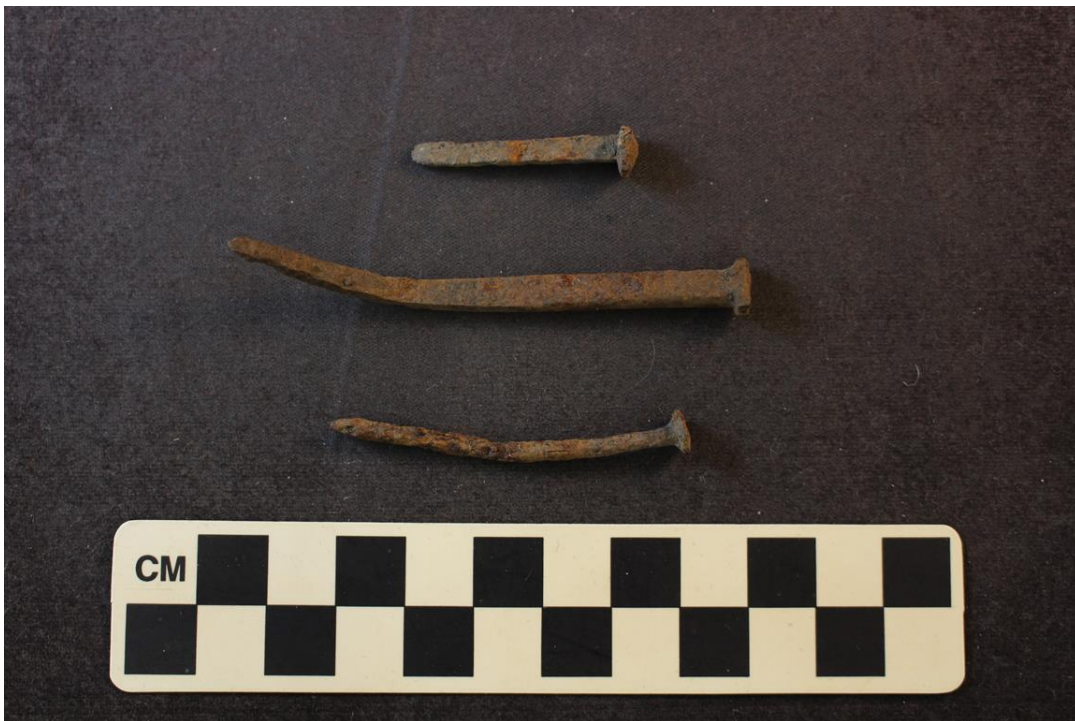
Image 19: (Top to bottom) wrought nail, machine cut nail, and wire nail.
